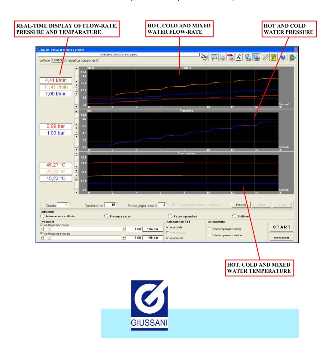
SETTING OF TEST PARAMETERS: STARTING PRESSURE, PRESSURE STEP AND STABILISATION TIME
