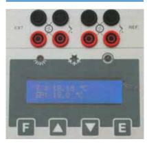
Panel with bushings for reference and sample probes
