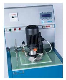
Fiberglass cover plate, side stand for probes to be calibrated and safety level switch
