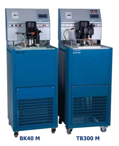
The **BK40 M** and **TB300 M** are thermostatic baths used for temperature probes calibration in the laboratory.
