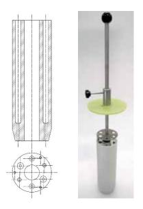
Both baths can be provided with equalizing blocks which enable improved stability and uniformity of the calibration zone.
