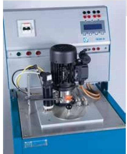
Stainless steel and Anticorodal cover plate, side support for probes to be calibrated and safety level switch
