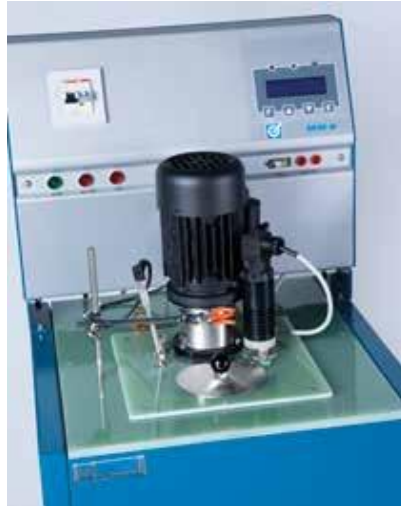
Fiberglass cover plate, side stand for probes to be calibrated and safety level switch
