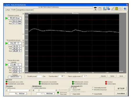
E) AQ2TB-EN12293 Software suitable to perform thermal cycle tests on multi-layer piping assemblies and fittings. The test consists to submit the device to temperature cycles with the passage of alternating hot and cold water.
