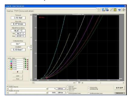
B) AQ2TB-KV-LAB Software for the evaluation of the pressure loss, caused by a device installed in a hydraulic plant, measuring the differential pressure  $\Delta P$  as a function of flow-rate.
