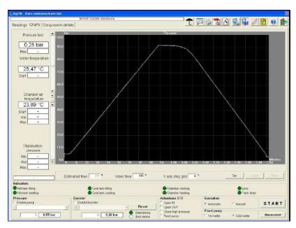
C) AQ2TB-PULSEAUT Software for performing water hammer tests and cycling pressure tests. The software allows to evaluate the strength and tightness of the component under test as a result of fast variations of supply pressure. It is possible to perform cycling pressure tests with water circulation (by hydraulic pump) and tests of resistance to water hammer without water circulation (by hydraulic booster).
