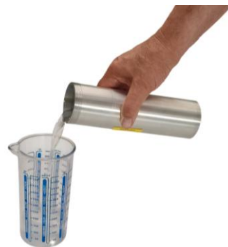
6. Drain the oil, clean the insert with paper towels, and fill in with the desired oil.
