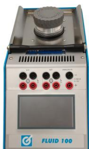
4. Once the insert is inserted, unscrew the cap and proceed with calibrations.
