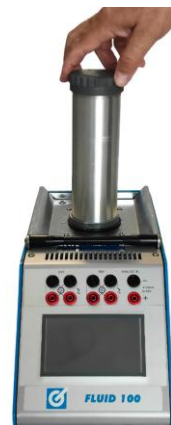
3. Screw the cap all the way down and place the insert into the calibrator.
