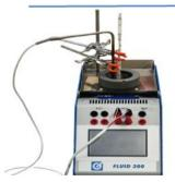
Fluids are equipped with adjustable holders support the probes under test or thermometers
