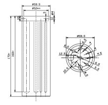
Perforated insert for Fluid H100 e 200 **Codice: 2D2846**
