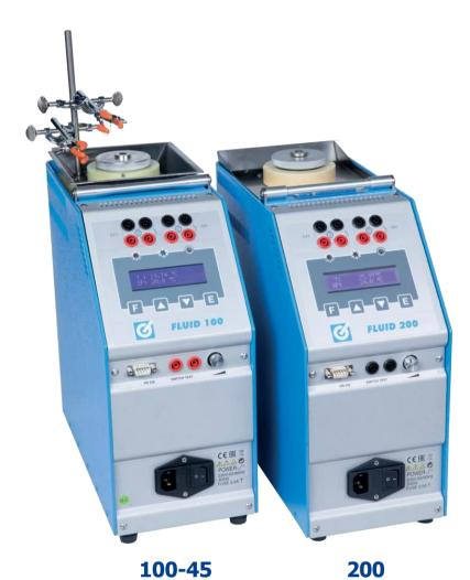
**FLUID** are portable thermostatic liquid calibrators used for checking thermocouples, platinum resistance and glass thermometers in the laboratory as well as in the field. It consists of an aluminium liquid bath whose capacity is about 400 cc and it is constantly kept homogeneous by a magnetic mixer whose speed is adjustable according to the viscosity of the fluid used.
