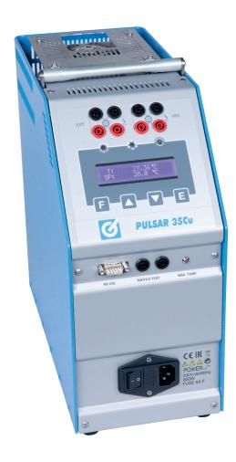
**PULSAR-35Cu** temperature calibrator is a compact instrument used to calibrate transducers, RTD and temperature-measuring sensors in the field and in the laboratory. The possibility to generate positive and negative temperature ramps makes it suitable for use in calibrating and testing thermostats.
