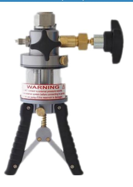
The portable Calibration Test Pumps **LPP 700** and **LPP 1000** are been designed for easy to use pressure calibration equipment "in the field", for testing pressure gauges, pressure switches and pressure transmitters. 10.000 PSI (700 bar) and 14.500 PSI (1000 Bar) can be reached in a simple way, using the "prime/high pressure" selector.
