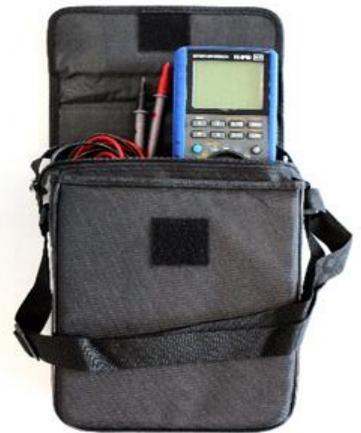
•The MPM-26 is the ultimate troubleshooting tool for electricians and process control professionals. It combines the functionality of a full-featured multifunction process calibrator with the power of a CAT III 1000 V, CAT IV 600 V safety rated digital multimeter
