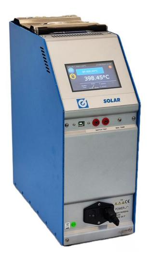
The new **SOLAR T** are portable thermostatic calibrators for laboratory and field testing of temperature, thermocouples and Pt 100 sensors. They consist of a tubolar vertical well with an internal ceramic element to isolate electrical parts and an interchangeable equalising block.
