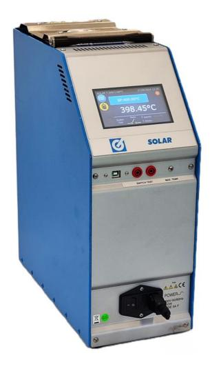
The new **SOLAR T** are portable thermostatic calibrators for laboratory and field testing of temperature, thermocouples and Pt 100 sensors. They consist of a tubolar vertical well with an internal ceramic element to isolate electrical parts and an interchangeable equalising block.
