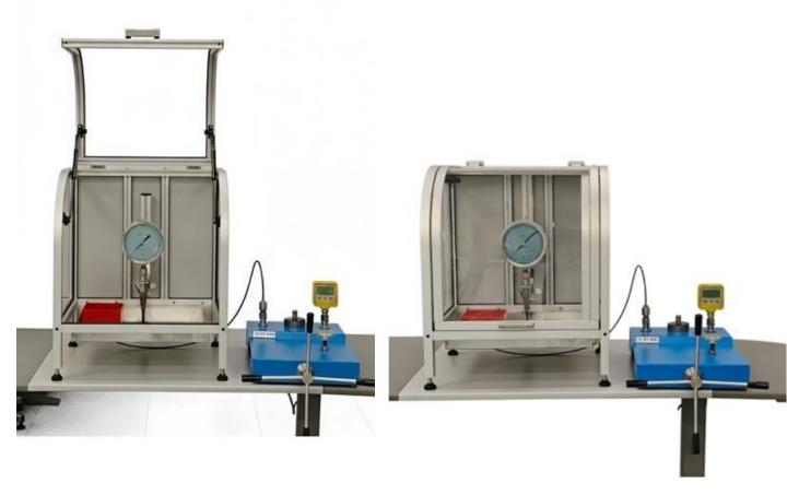
**Protection Safety Guard** was specifically designed to guarantee **maximum operator safety** during the execution of high-pressure testing and calibration that involve the risk of bursting.
