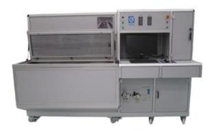
Models are available with horizontal test chamber with dimensions in length from 800 mm up to 1,600 mm (see above), or with vertical test chamber with heights up to 1,600 mm (see to the side).
